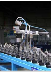
alkitronic® CLV operating in a preassembly and final assembly workstation. Remote controlled continuous tightening in semi-automatic operation.
